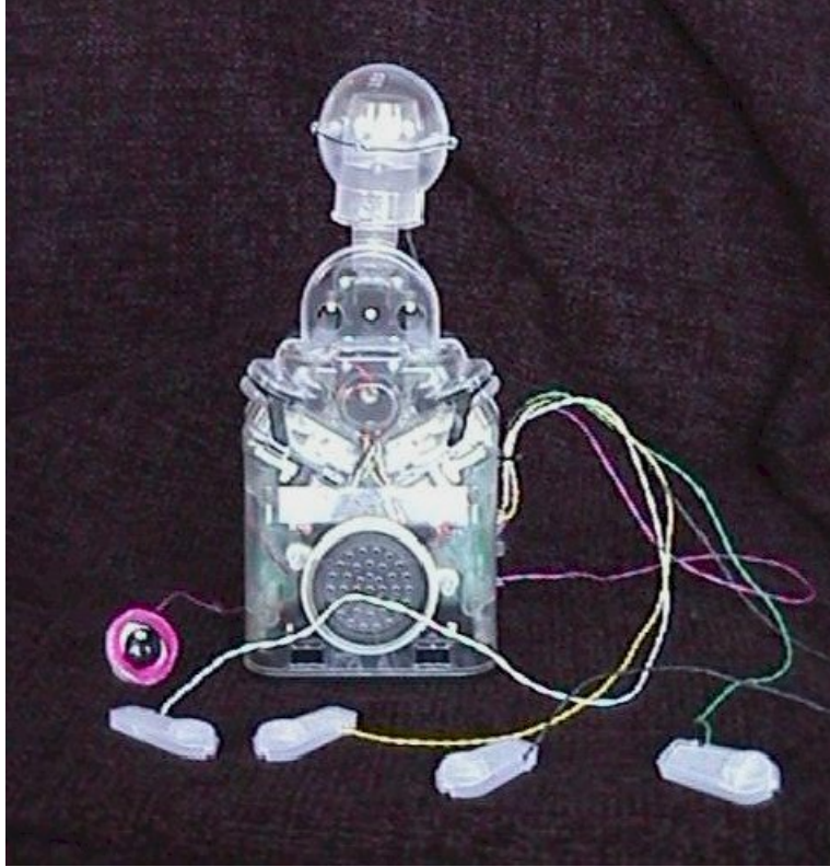
Figure 1. Technology without personality. The “chassis” for the Barney interactive character, with hand, feet, and eye sensors attached.
