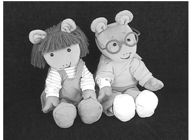
Figure 1. ActiMates D.W. and ActiMates Arthur. Children respond to the character's speech and gestures by squeezing sensors located in the hands, feet, ears, and watch (visible on right arm).
